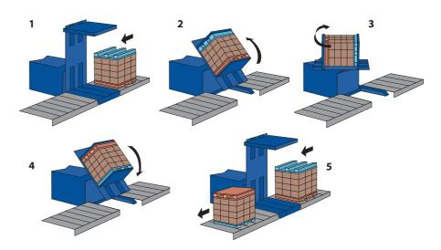
The RR can also be sited 'off-line'. The picture to the left shows how loads of boards which need turning can leave the main conveyor route, enter the RR and then return to it after inversion.
